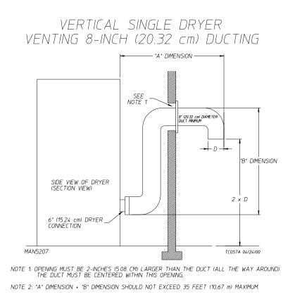
When single 8-inch (20.32 cm) vertical venting is used (refer to the **illustration below**), the ductwork from the dryer to the outside outlet <u>cannot</u> exceed 35 feet (10.67 meters) in total length. This calculation of 35 feet (10.67 meters) compensates or allows for the use of a maximum of three (3) elbows including the 180° (turned downward) outside outlet.
